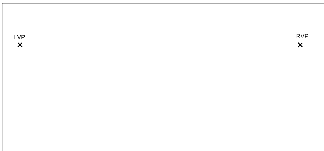
Figure 9-1: Draw a horizon line across the paper, about \frac{2}{3} the paper from the bottom. Make sure that the line is horizontal. Then make two vanishing points, one on each end of the horizon (the left and right vanishing points, LVP and RVP).
